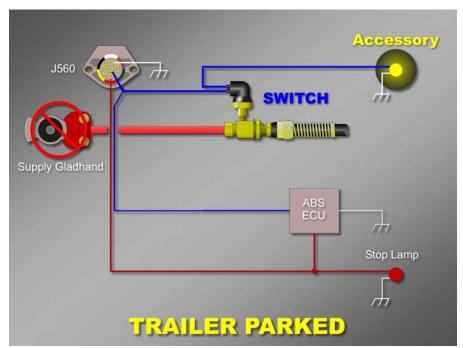
As illustrated by this schematic, the switch is installed in a branch of the blue circuit supplying power to the accessory device. By tapping into the air line from the supply gladhand, the switch
