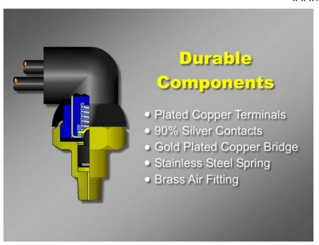
This sectional view illustrates the operation of the switch, shown in the parked or "accessory on" position. Air applied to the 1/8 pipe thread port will act on the piston to raise the copper bridge off of the terminal contact, breaking the circuit.
