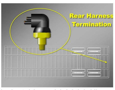
... at the rear harness termination, ... or any other location that the air and wiring are accessible.
