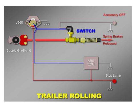
When the parking brakes are released by pressurizing the supply gladhand, the switch reads the line pressure, and opens the
