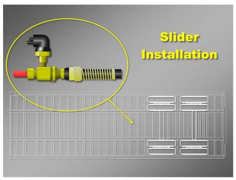
The optional anchor tee fittings for 1/2" and 3/8" O.D. tubing provide easy installation at the slider hose connection, as shown in the previous schematic.
