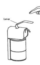
7. Depress the lever vigorously 4-5 times to prime the unit.
