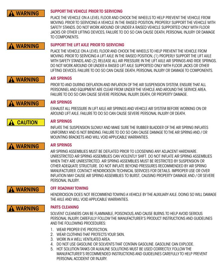
DO NOT USE HOT SOLUTION TANKS OR WATER AND ALKALINE SOLUTIONS TO CLEAN GROUND OR POLISHED PARTS. DOING SO WILL CAUSE DAMAGE TO THE PARTS AND VOID APPLICABLE WARRANTIES.
