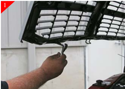
1 Start with removing the (12) 8mm. Bolts from the back-side of the stock grille shell as shown. Grille shell will be free at this point. With shell removed tape the face of the grille shell to protect during install.
