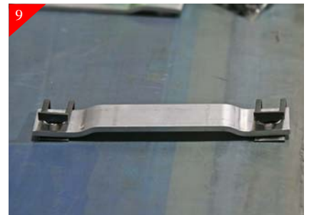
9 Next place the supplied u-clips on the middle support bracket as shown above.
