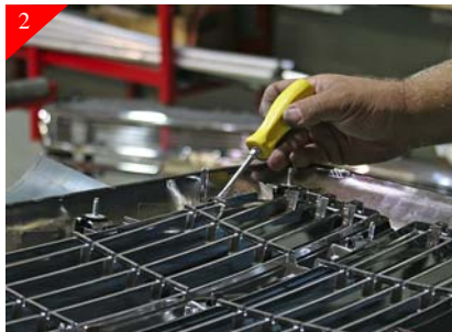
2 Un-snap plastic inserts as shown. It maybe necessary to use a regular screwdriver to aid in the release of the clips.
