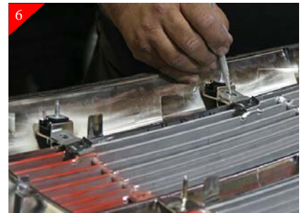
6 Then place the top portion of the billet grille into opening and center. Attach the brackets using the supplied U-clips and #8 x 5/8" Phil pan head screw. Next mark the locations of the holes where it meets the stock grille
