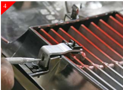
4 Place bottom billet grille into opening and center. Next attach the brackets to the billet grille using #8 x 5/8" Phil pan head screw. Then using a scribe mark the hole locations where the bracket meets the stock grille as shown above.
