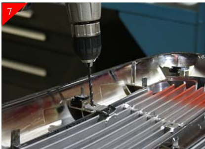
7 Then drill a 3/16" hole in the just marked locations.
