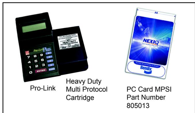
**FIGURE 14 - NEXIQ (MPSI) PRO-LINK TOOL**
