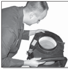
Inspect the engine air cleaner.
