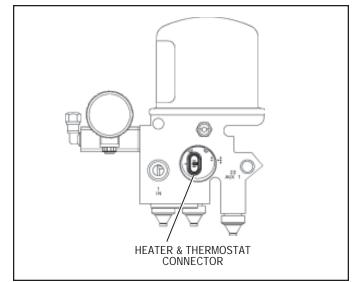
FIGURE 4 - AD-IS<sup>®</sup> AIR DRYER AND RESERVOIR SYSTEM HEATER AND THERMOSTAT CONNECTOR
