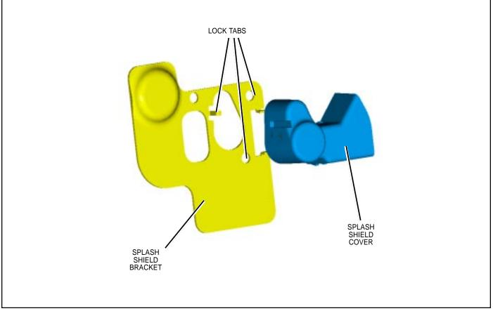
FIGURE 6 - SPLASH SHIELD BRACKET AND COVER - (EXPLODED VIEW)
