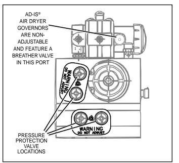
FIGURE 5 - PRESSURE PROTECTION VALVE LOCATIONS
