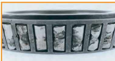
Rapid and deep spalling caused by unusually high stresses. Full race width fatigue spalling is caused by heavy loads creating a thin lubricant film and possible elevated temperatures.
