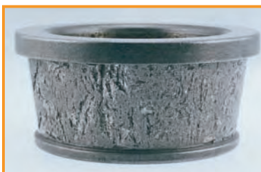
Rapid and deep spalling caused by unusually high stresses. Full race width fatigue spalling is caused by heavy loads creating a thin lubricant film and possible elevated temperatures.
