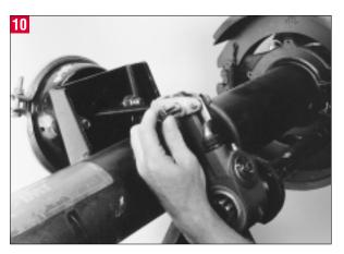
Once the clevis is properly aligned with the slack adjuster, insert both the large and small clevis pins and secure with the cotter pins supplied.
