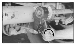
7. Once the linings have been replaced and the brake drum installed, rotate the hex extension clockwise until the brake linings contact the brake drum.
