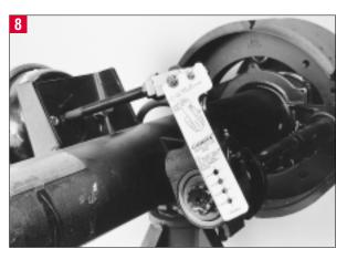
After threading the 1-1/4" collar nut onto the clevis housing, place the template over the large and small clevis pins as shown above.
