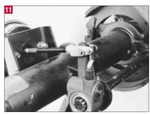
Fully apply the brakes and allow the chamber push rod to travel its maximum stroke. Clearance must exist between the slack adjuster and all adjacent chassis components. Release the brakes.
