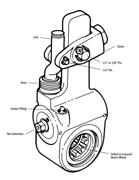
Figure 1 - Gunite Slack Adjuster
