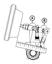
Figure 4 – Measuring Maximum Stroke
