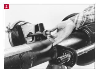
When installing a Gunite slack adjuster with a collar lock clevis, place the 1-1/4" collar nut on the push rod against the 15/16" jam nut. Next thread the 3/4" hex nut onto the push rod.
