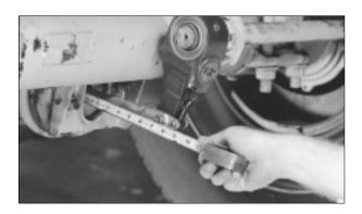
**9.** Using a ruler, measure the distance from the face of the air chamber to the center of the large pin in the clevis (A) (see fig. 14).
