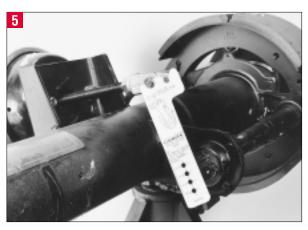
Once the clevis has been installed on the threaded push rod, install both the large and small clevis pins. Now position the installation template over both the large and small clevis pins.
