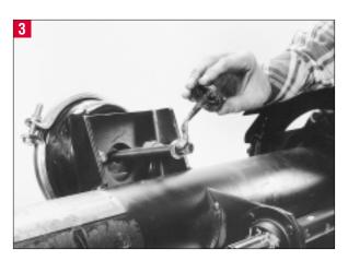
Apply anti-seize to the chamber push rod threads before installing the new clevis. Also apply anti-seize to the camshaft at this time.
