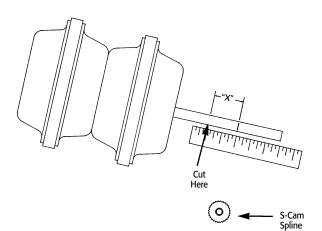
Figure 13 - Cutting the Push Rod
