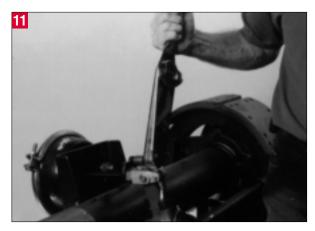
Once the 1-1/4" collar nut has been properly tightened to the clevis, tighten the 15/16" jam nut against the collar lock nut using 40 to 50 ft lbs of torque.
