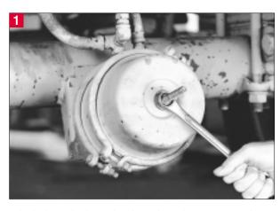
Block the vehicle's wheels. If the axle is equipped with spring brakes, manually cage the brakes following the manufacturer's recommended procedures.
