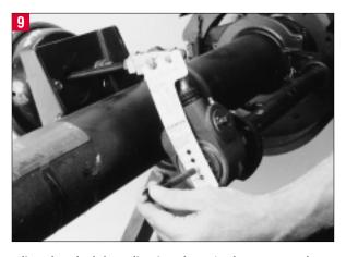
Align the slack by adjusting the 3/4" hex nut on the push rod until the appropriate centering hole on the template aligns with the center hole on the camshaft. The template is provided with centering holes for 5, 5.5, 6 and 6.5 inch slacks.
