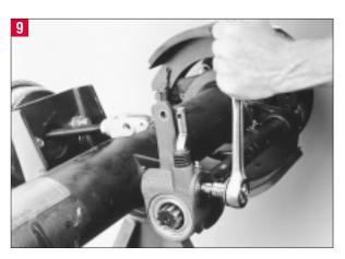
Apply anti-seize compound to the camshaft, install the slack adjuster and adjust the position of the slack using the hex extension. Adjust the slack until the holes in the slack housing align properly with the corresponding holes in the clevis.
