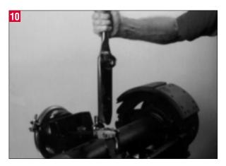
Using a torque wrench, tighten the 1-1/4" collar nut to the clevis using 40 to 50 ft lbs of torque.
