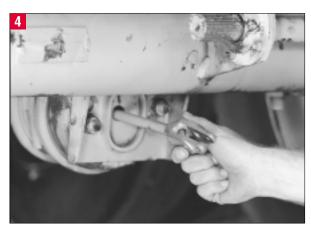
When installing a Gunite slack adjuster with a threaded clevis, install the new clevis on the push rod in the same location as the clevis which was removed. Do not tighten the jam nut at this time.
