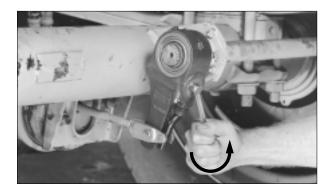
**8.** Back-off the slack adjuster by rotating the hex extension 1/2 turn counterclockwise. A ratcheting sound will be heard. This will provide running clearance between the lining and the drums braking surface.
