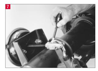
Before attaching the 1-1/4" collar nut to the clevis, check to make sure the threaded push rod is fully engaged in the 3/4" hex nut. If the push rod does not have full engagement, a new push rod must be installed and cut to length. Refer to the section on cutting a new pushrod to length in the service manual.
