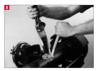
Tighten the jam nut against the clevis housing using 40 to 50 ft lbs of torque. If you do not tighten the jam nut now, it will allow the clevis to rotate freely and change the position of the clevis resulting in an improper installation.
