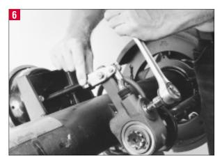
Using the hex extension and a wrench, adjust the slack so that the collar nut aligns with the threaded area of the clevis.
