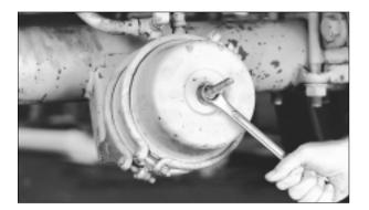
If the vehicle is equipped with spring brake chambers, manually cage the spring brakes following the manufacturer's recommended procedures.
