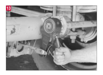
Pre-adjust the brakes by rotating the hex extension clockwise until the brake lining contacts the brake drum. Back the slack adjuster off by rotating the hex counterclockwise 1/2 turn. Backing off a new slack adjuster may require up to 50 ft lbs of torque. A ratcheting sound will be heard when backing the slack off.
