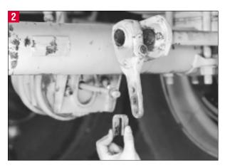
Remove the existing clevis and slack adjuster. Keep the existing mounting hardware. Do not remove the clevis jam nut.
