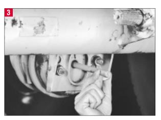
Apply anti-seize to the chamber push rod threads before installing the new clevis.
