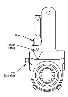
Figure 6 – Lubrication Points
