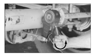
Using a 7/16" wrench or socket, rotate the hex extension counterclockwise. You should have at least 15 ft lbs resistance and a ratcheting sound will be heard as the hex extension is rotated.
