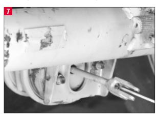
Inspect the clevis installation to make sure that the threaded push rod extends no more than 1/16" past the end of the opening of the clevis in the clevis housing. If the push rod extends more than 1/16" past the clevis housing, the clevis must be removed and the push rod cut to the proper length.
