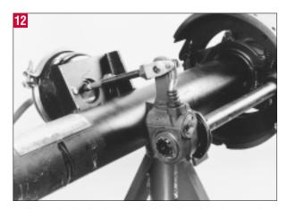
Fully apply the brakes and allow the chamber push rod to travel its maximum stroke. Clearance must exist between the slack adjuster and all adjacent chassis components. Release the brakes.
