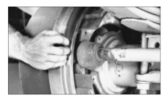
Only back off the adjusting hex enough to allow the drum to clear the lining. Remove the brake drum.
