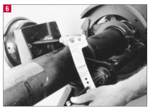
Align the clevis on the threaded push rod until the appropriate centering hole on the template aligns with the center hole on the camshaft. The template is provided with centering holes for 5, 5.5, 6 and 6.5 inch slacks.
