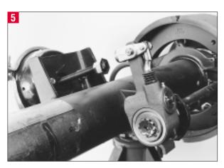
Install the slack onto the camshaft using the original mounting hardware.
