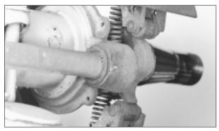
5. After the brake drum has been removed; rotate the hex extension clockwise until the cam turns over. This will allow the brake rollers to be in the release position.
