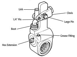
Figure 9 - Location of Clevis Pins, Hex Extension & Boot
