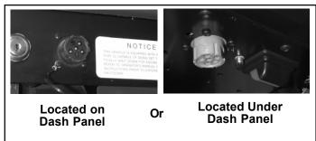
(Note: An adapter is required when the vehicle has a 6-pin connector.)
